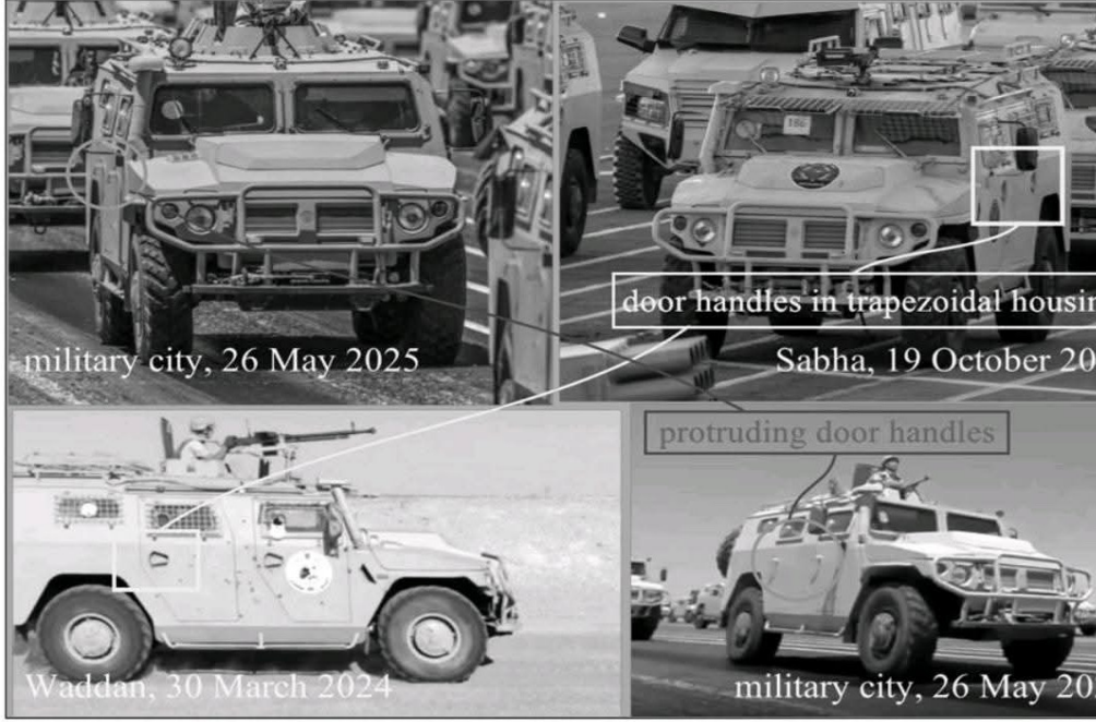
Figure 24.F.4 Tigr-M and Tigr SBM VPK-233136 (five-door version)
